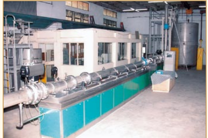
Experimental set-up to measure fluid flow in closed pipes in the range 0.1 - 60 m 3 /h by determining the amount fluid collected over a period of time. It provides a platform for evaluating the performance of the flow measuring devices
