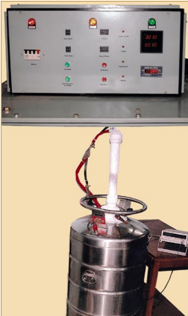
Set-up for measurement of 1000 A current carrying of 30 mm diameter 30 cm long Bi2223 tube electrode at liquid He temperature
