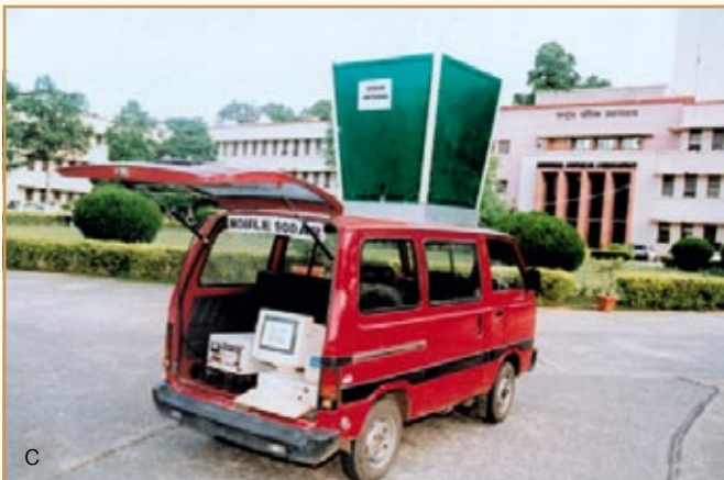
Monostatic sodar system presents atmospheric pictures on round-the-clock basis. This makes it an extremely useful device to map atmosphere continuously. Photograph shows (a) Complete system electronics developed at NPL, which can be housed in a vehicle for mobile operations. (b) Phased array antenna for beam steering developed at NPL. This antenna is enclosed in a hexagonal shield, and (c) Hexagonal Doppler sodar shield mounted on the top of a vehicle for mobile operation
