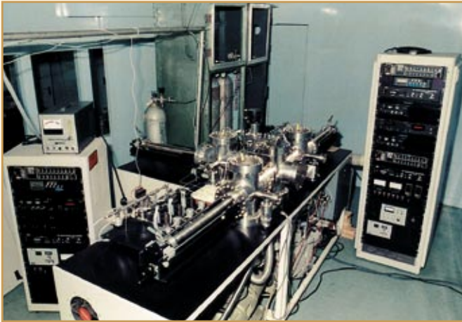
Three chamber PECVD system used for fabrication of p-i-n a-Si:H layers for solar cells
