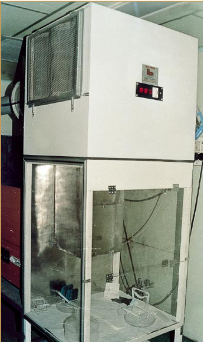
Diffusion furnace used for phosphorous-diffusion in 100 mm diameter or 100 mm x 100 mm size Si wafers for creation of n + -p junction for silicon solar cells
