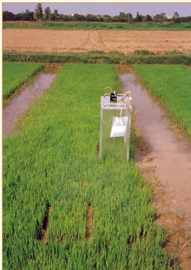
Static box technique used for air sampling in the paddy fields of the IARI, New Delhi
