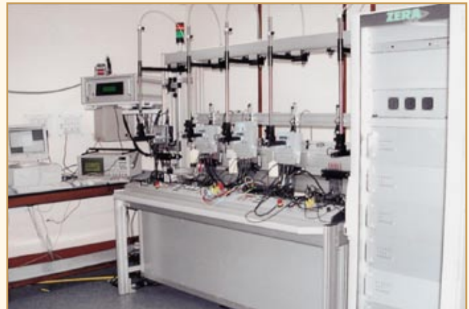
Bench for the calibration of power/energy meters (maximum five at a time) using precision comparator and stable power/energy source
