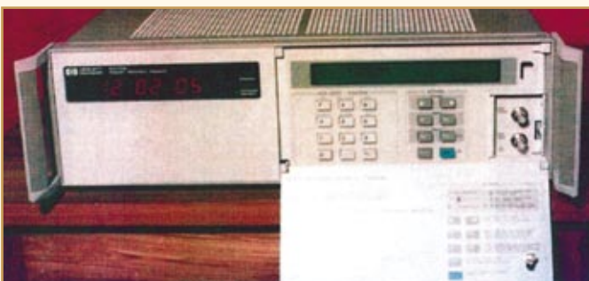
NPL has been maintaining Indian Standard Time (IST) through the cesium atomic clock (internationally accepted primary standard for time) since 1974. Time scale of NPL is maintained within few nanoseconds with respect to Universal Coordinated Time (UTC)
