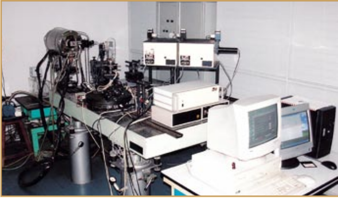
Variable temperature blackbody is the primary standard for establishing the scale of optical radiation with reduced uncertainty in the measurement of photometric parameters
