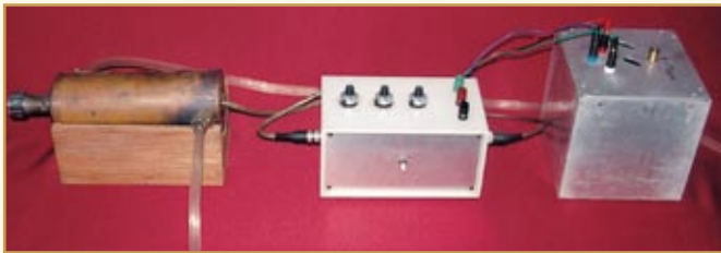
Power mount of a commercial power meter has been modified by NPL in 1985 serves as a Primary Standard of High Frequency (HF) voltage in the frequency range 1 MHz to 1 GHz. This mount is based on calorimetric principles which uses RF-DC substitution technique for measurement of HF voltage
