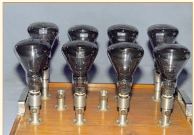
A set of luminous intensity standard lamps which are used for maintaining the base unit 'candela' and for calibrating sources for luminous flux as well as for quality control of lamp and lighting products
