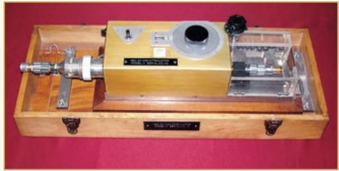
A 30 MHz Waveguide Below Cut Off (WBCO) attenuator of range 60 dB developed by NIST, USA, and established at NPL in the year 1975 serves as the primary standard of attenuation
