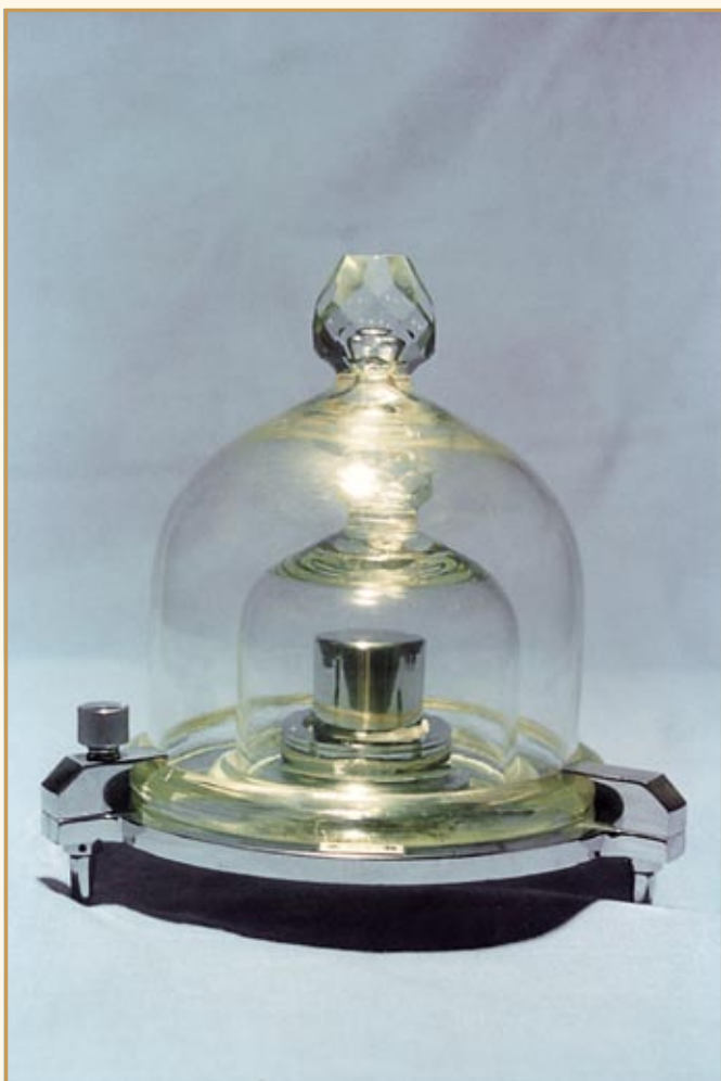
The National Prototype Kilogram is Copy No. 57 of the international Prototype Kilogram (base unit of mass), which serves as the Primary Standard of Mass of the country. It is traceable to the international standard and is kept under the custody of NPL
