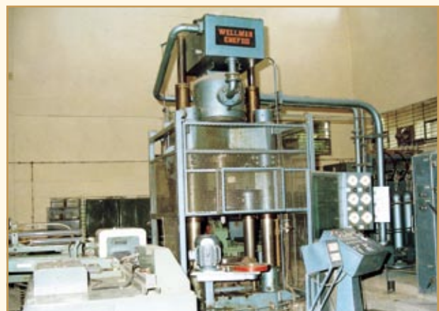
500 tonne vertical hydraulic multipurpose instrumented press set-up in 1980 under Colombo Plan Assistance Programme and being used for developing ferrous, non-ferrous and composite components employing hot extrusion and near-net shaped cold/warm forging
