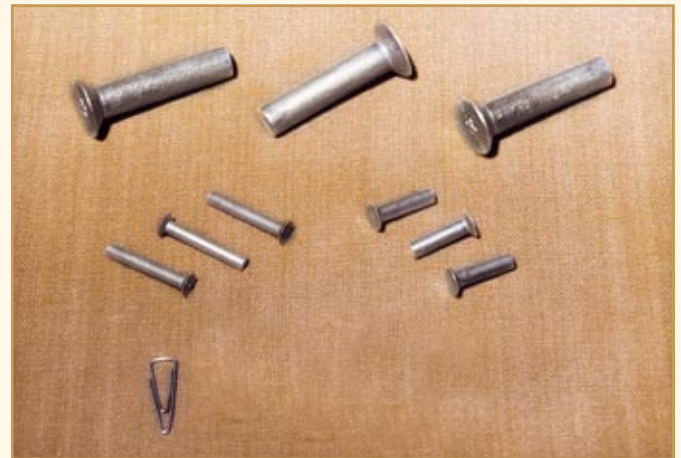
Aerospace grade Al-alloy rivet wires developed jointly with HAL under the indigenization programme for aerospace industries
