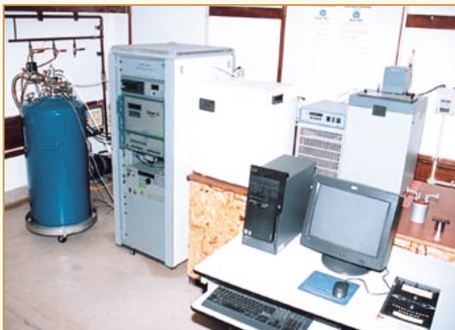
Experimental setup for realization of the primary standard of resistance based on integral Quantum Hall Effect
