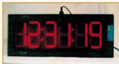
Innovative time service via telephone line (Teleclock Service) for common users of time. One can get access to IST within a second or two with the help of Teleclock receivers developed by NPL. Few models of Teleclock receivers available in the market are shown
