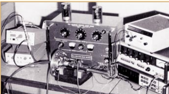
Primary standard set up for High Frequency Voltage Prior to 1985 was based on indigenously developed bolometric mount in the frequency range 10 MHz to 1 GHz
