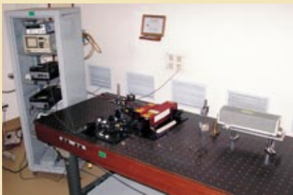
Iodine frequency stabilized He-Ne Laser, used for practical realisation and dissemination of unit 'metre'
