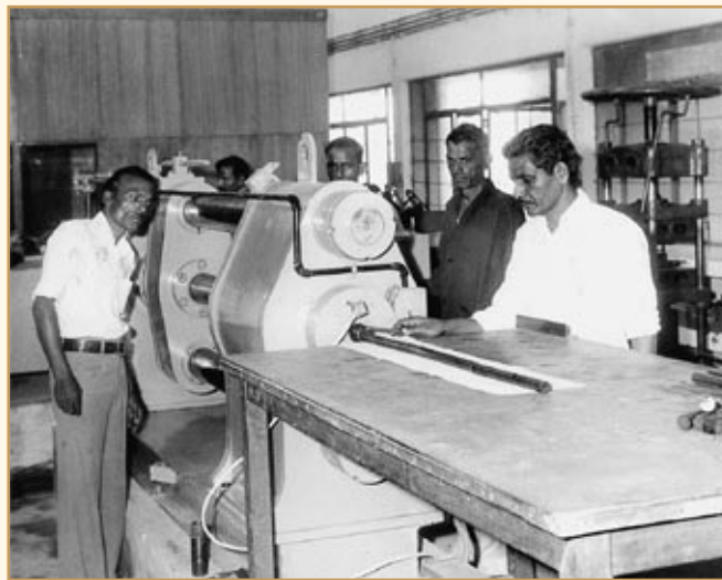
A view of the carbon pilot plant showing production of cinema arc carbons by NPL's patented process of simultaneous extrusion
