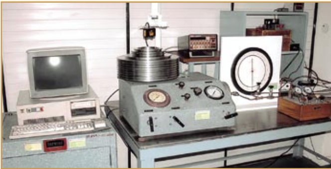
Primary pressure standard in the pneumatic pressure range in gauge mode - Controlled Clearance Piston Gauge (CCPG). This instrument is used to calibrate instruments which are used for measuring pressure in LPG and natural gas cylinders, tyre pressure of automobiles etc.
