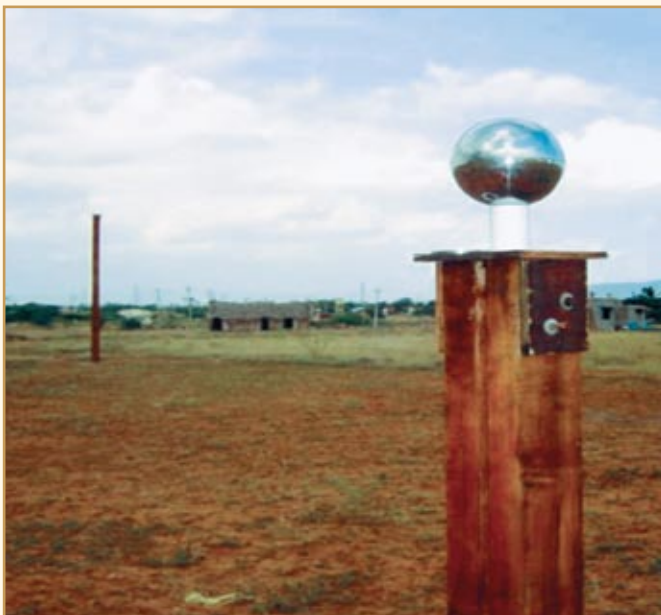
Experimental setup for measuring AC and DC components of the Global Electric Circuit (GEC) formed by the Earth, the ionosphere and the atmosphere in the study of ionospheric dynamics
