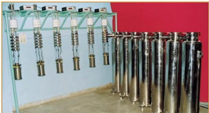
7 Tesla (50 mm bore) superconducting magnets along with support system and superinsulated liquid helium cryostats
