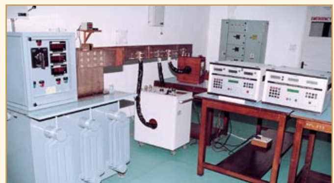
Bench for the calibration of Current Transformers (CTs) for a current ratio from 5 A/1 A, 5 A to 5000 A/1 A, 5 A at 50 Hz
