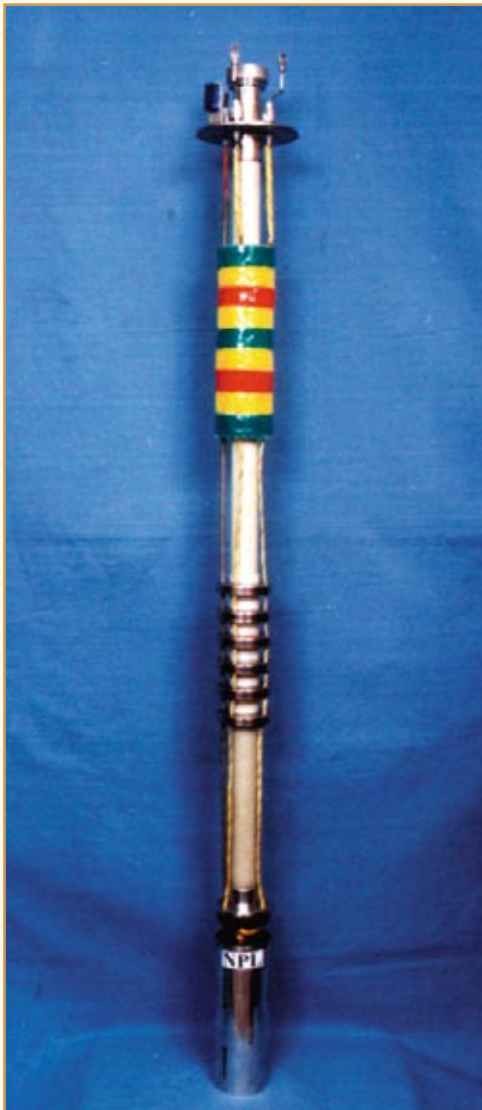
A light weight, compact 3.5 Tesla Insert type superconducting magnet
