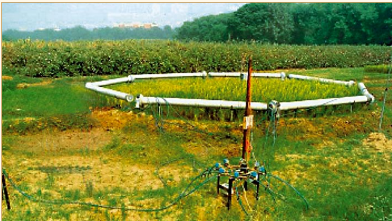
Enhancement of CO 2 in the atmosphere can effect the agriculture output. An automatic facility to enhance CO 2 in the open air was developed by NPL in 2000 and installed at IARI campus , New Delhi, to study response of crops to elevated levels of CO 2
