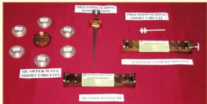
Indigenously designed and developed quarter wave (QW) short circuits and precision waveguides (Primary standards of impedance) and standard mismatches (Transfer standards of impedance)
