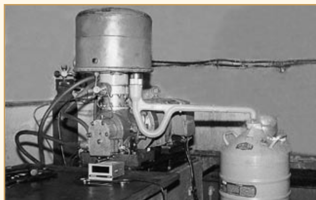
The first NPL developed Stirling cycle based liquid air plant producing 3-4 litres of liquid air per hour
