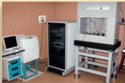
Automatic Gauge Block Interferometer, the first link between definition of unit metre and length measuring artifacts - Gauge Blocks upto 300 mm
