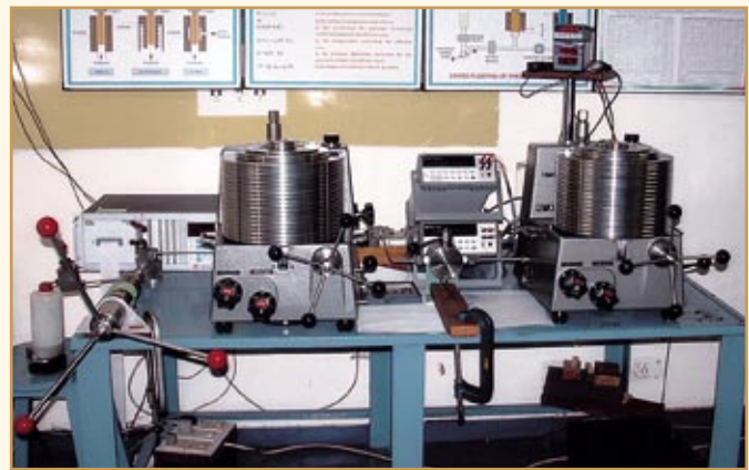
Method of crossfloating of two different secondary standards by which all pressure calibrations are carried out. This becomes an indispensable for modern development and production processes
