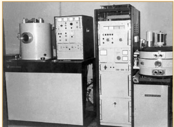
A-500 thin vacuum coating plant (left) and VZK-550 Sputtering plant
