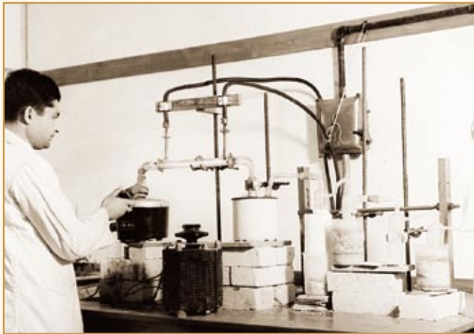
Set-up for thermal decomposition of silicon tetra iodide on tantalum wire for obtaining poly-Si
