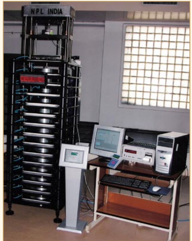
Automated load cell calibrator designed, developed and fabricated at NPL for Regional Reference Standard Laboratories (Ministry of Consumer Affairs) for the calibration of load cells used in commodity weighing in order to ensure consumer protection
