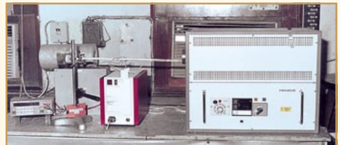
Experimental set-up for comparison calibration of noble metal thermocouples using high temperature horizontal furnace in the range 100\text{ }^{\circ}\text{C} - 1000\text{ }^{\circ}\text{C}
