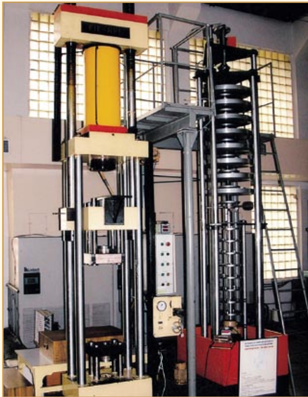
Hydraulic multiplication machine designed and developed at NPL to calibrate force transducers (proving rings, load cells, Amsler boxes etc.) upto 1000 kN, which are used in the verification of testing machines
