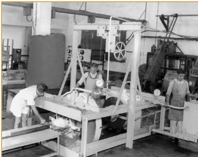
A view of carbon pilot plant showing 200 tonne hydraulic extrusion press in operation for extruding green carbon mix into carbon electrodes
