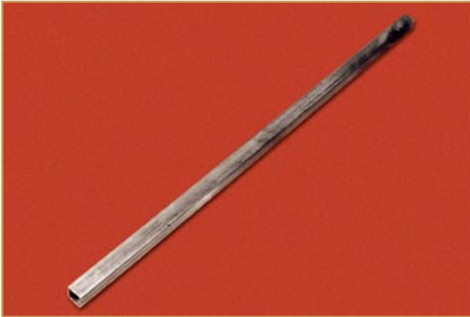
Mg-alloy square extruded tube developed for VSSC for its proposed use in PSLV under the weight reduction programme
