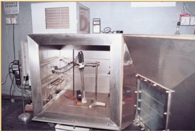
Reference (National) Humidity Standard [An aspirated psychrometer] used to calibrate hygrometers in the range of 15% to 95% Relative Humidity
