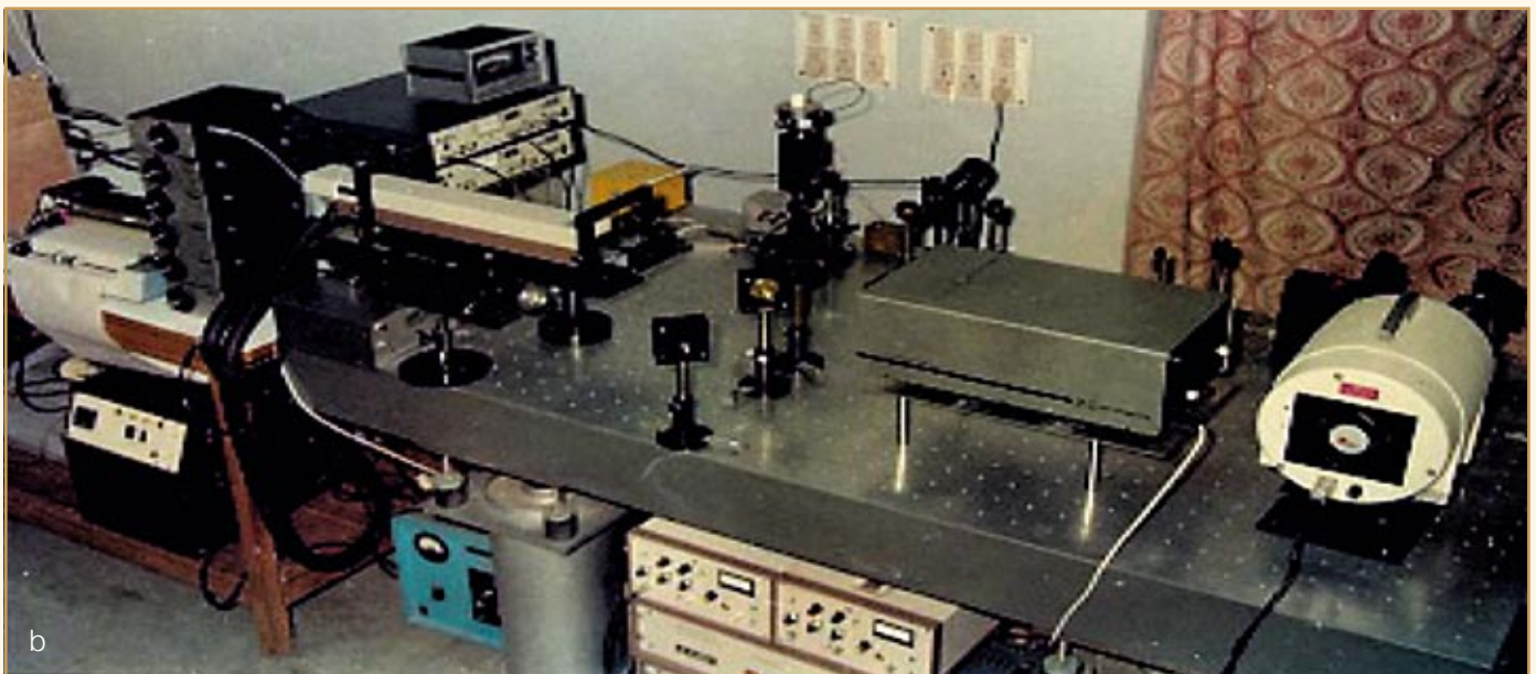
To study long-term changes in Antarctic environment, NPL installed several experiments at the Indian Antarctic station, Maitri. Photograph shows (a) Monostatic acoustic sounder and 28 m tower mounted at Maitri and (b) Laser Heterodyne System mounted inside the laboratory
