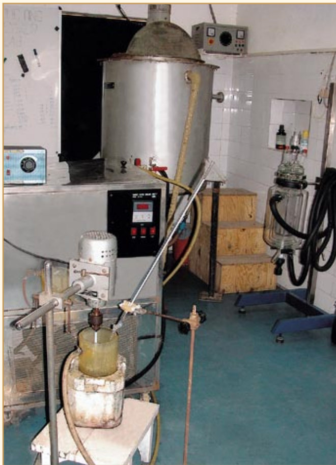
Double walled stainless steel and reactor assembly for the synthesis of conducting polymers
