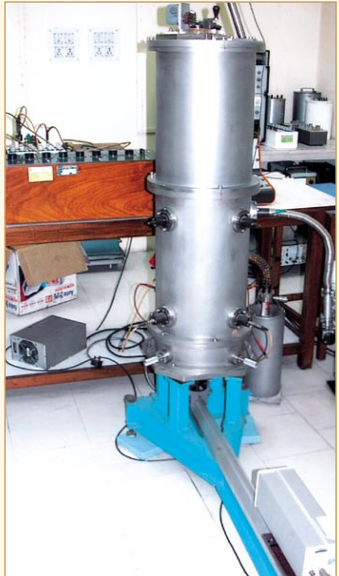
Primary standard of capacitance, calculable cross capacitor, established at NPL in collaboration with NPL, UK in 1980
