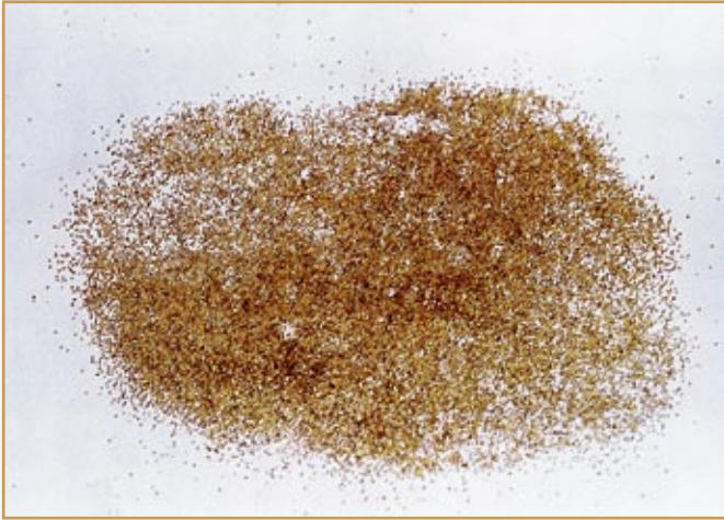
Single crystals of synthetic diamonds synthesized using 200 tonne cubic press
