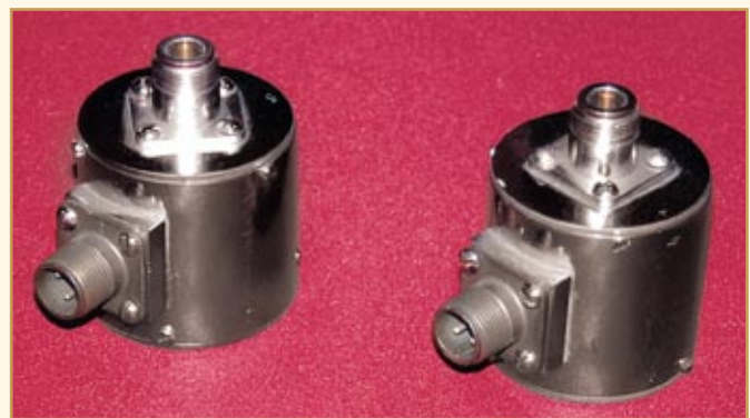
Primary standard of LF voltage and current, Multi Junction Thermal Converters (MJTC) is based on thin film technology (1 V to 3 V, 3 mA to 10 mA, 10 Hz to 1 MHz). These thin film MJTCs have improved frequency response
