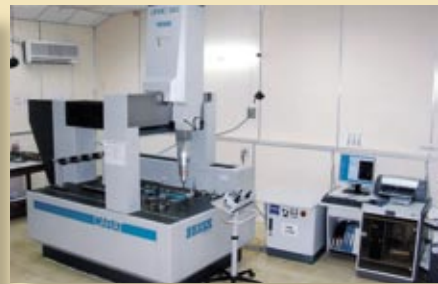
Three Dimensional Coordinate Measuring Machine (850 mm x 1200 mm x 600 mm), used to disseminate traceability to various standard artifacts, and instruments of industrial dimensional metrology. It is capable of measuring profiles, curvatures, angularity, flatness, deviation from roundness etc.
