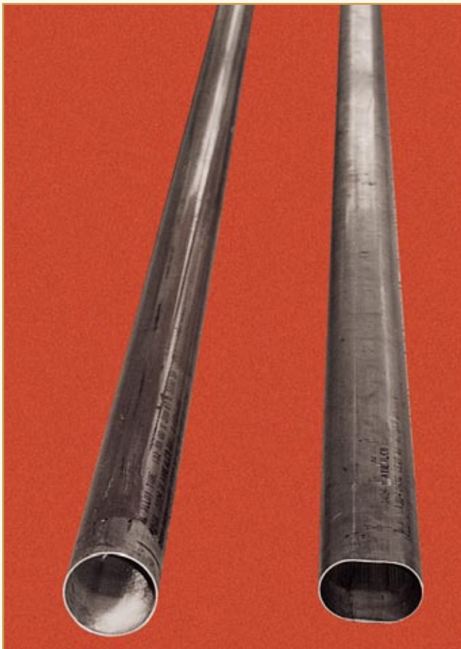
Oval shaped Al-alloy skid landing gear tubes developed for HAL for their use in ALH under weight reduction programme
