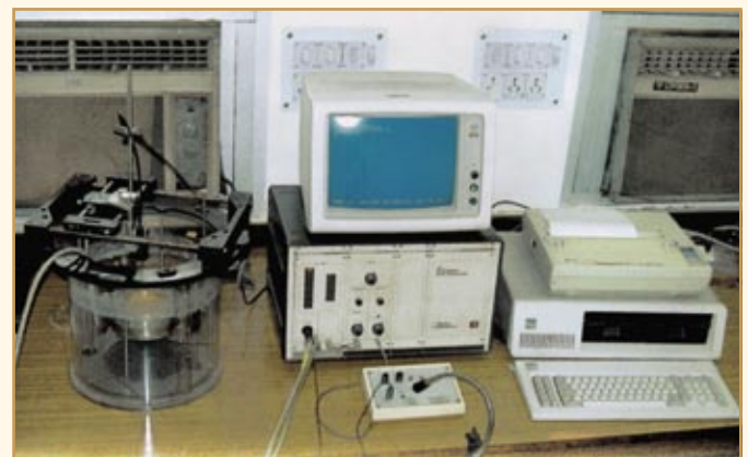
Experimental set-up for the calibration of ultrasonic medical equipment
