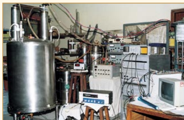
A high homogeneity superconducting magnet with room temperature bore cryostat integrated with NMR spectrometer (developed for the first time in India)
