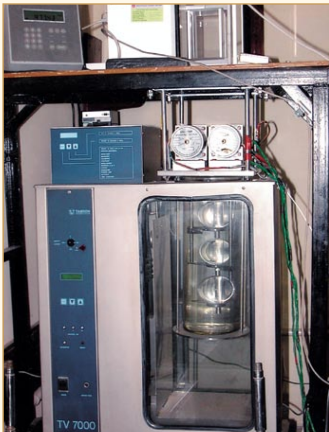
The set-up for solid density standard is a computer controlled fully automatic solid density measurement facility using hydrostatic weighing system. With this facility primary solid density standard traceable to the national standard of mass and density of pure distilled water has been realised
