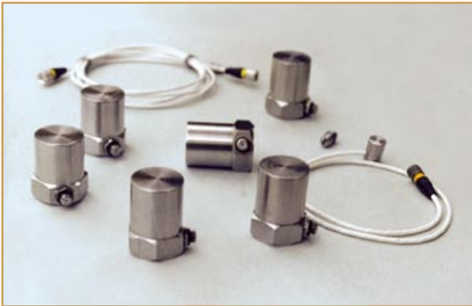
Piezoelectric accelerometers developed at NPL for shock (1 Hz to 20 KHz) and vibration (upto 3000 g) measurements. These are extensively used in defence and space applications
