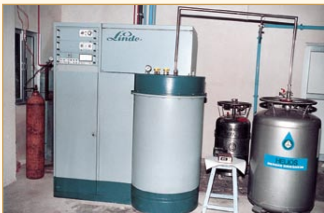
Helium liquefier with production capacity of 20 litre/hour (with precooling)
