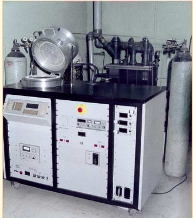
Plasma Enhanced Chemical Vapour Deposition (PECVD) system for giving silicon nitride AR coating to silicon solar cells
