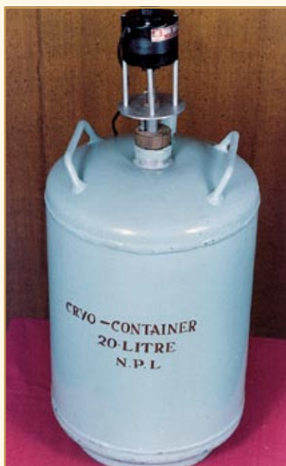
Superinsulated cryo-container (20 litre capacity) with liquid nitrogen transfer pump
