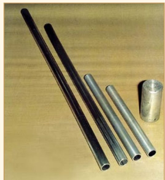
Aerospace grade MMC tubes, as compressive strut members for INSAT under weight reduction programme
