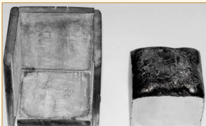
Reusable graphite crucible used a number of times to grow multicrystalline silicon ingots
