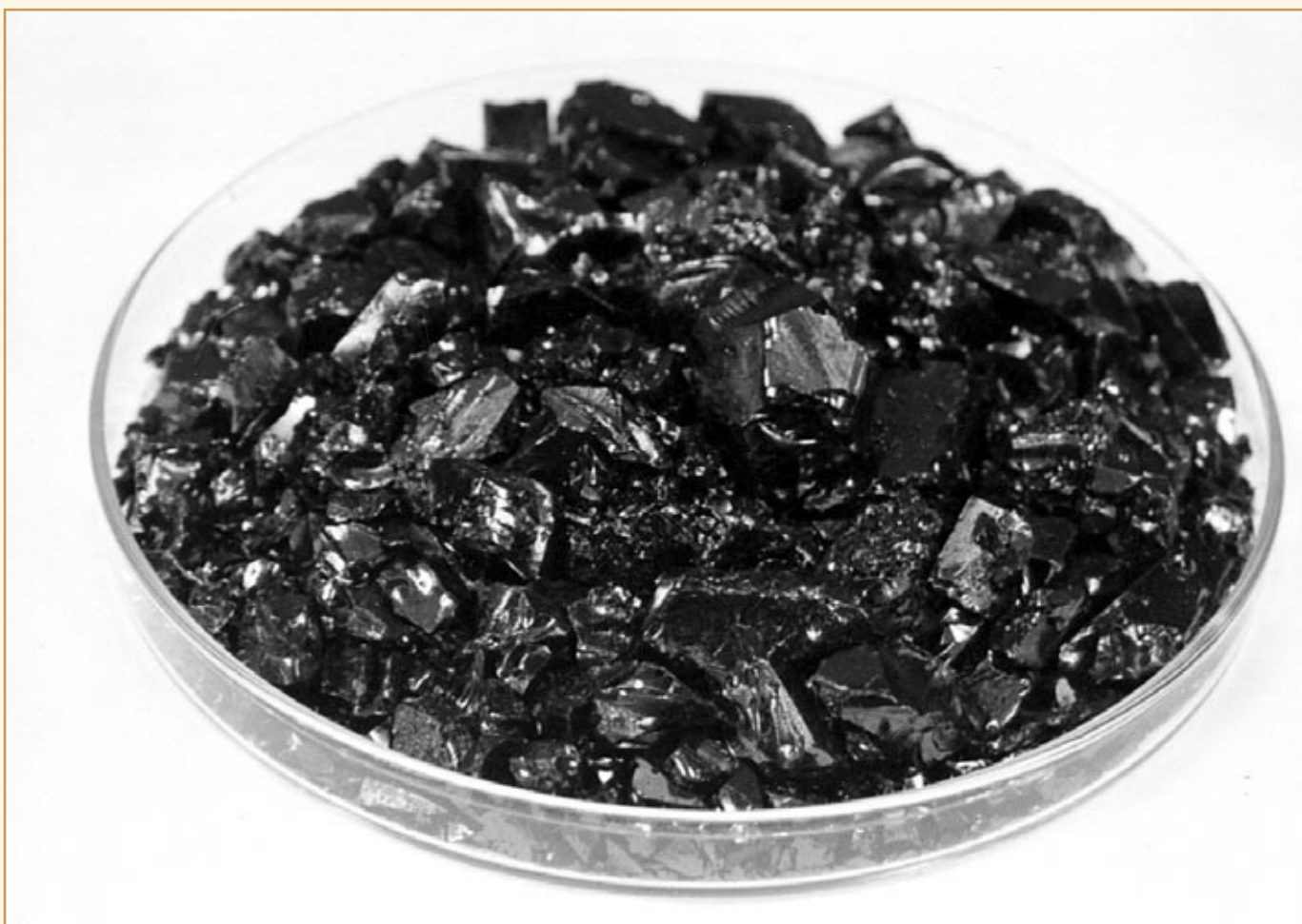
A sample of QI-free impregnating grade coal tar pitch developed at NPL by the state-of-the-art process. The pitch is used extensively for densification of graphite electrodes, carbon-carbon composites and also used as a precursor for carbon fibres, supreme quality needle coke, high density high strength graphite etc
