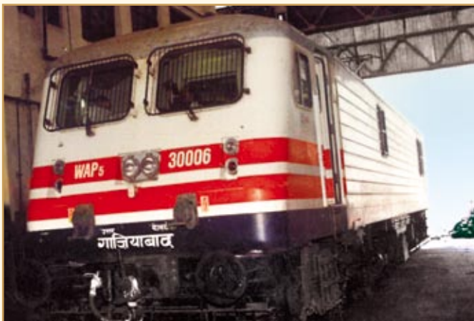
One of the Railway engine bogies imported by Indian Railway from M/s. ABB through their local representative M/s. ADTRANZ, India, was tested using strain and deflection measurements in real time between Delhi and Howrah at a few strategic points for the performance evaluation as per IR01-26.0 & IR01-27.0 standards
