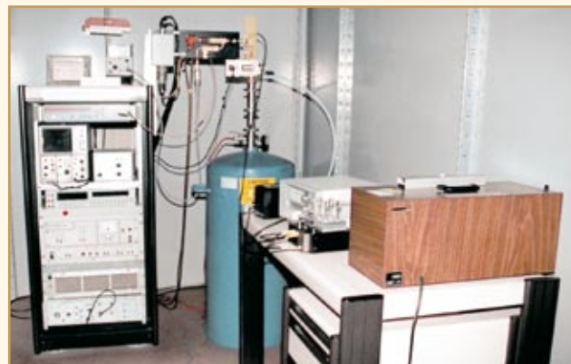
Experimental setup of Josephson Series Array Voltage Standard (JSAVS), as primary standard of volt (at 1 volt level)
