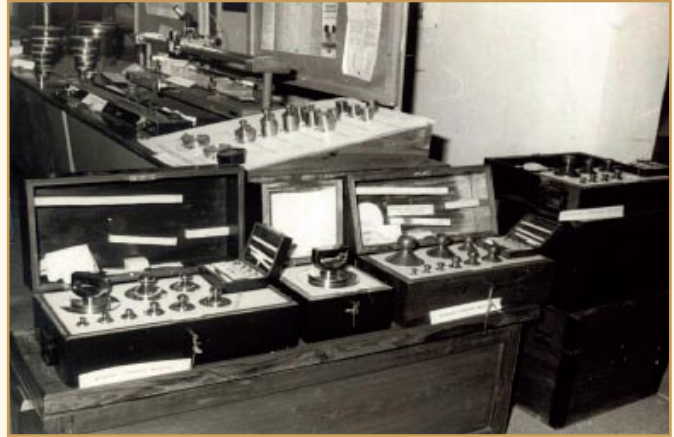
Standard weights and measures, designed by NPL and manufactured by the Government Mint, for the use of Legal Metrology Departments
