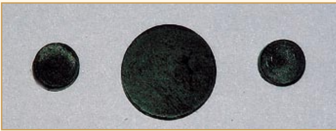
cBN polycrystalline composites synthesized using 200 tonne cubic press
