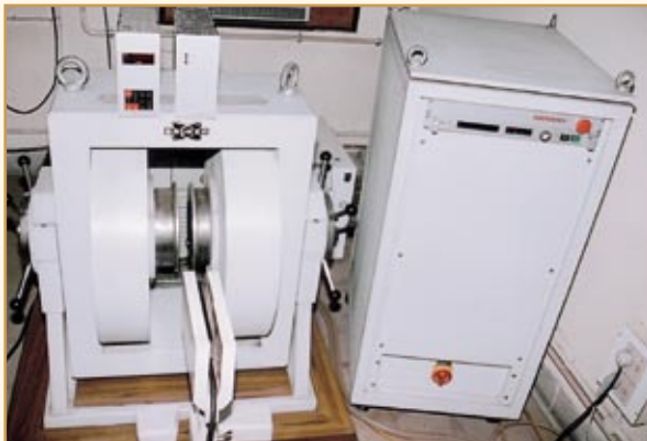
Experimental setup for the precise measurement of magnetic field using NMR Gaussmeter
