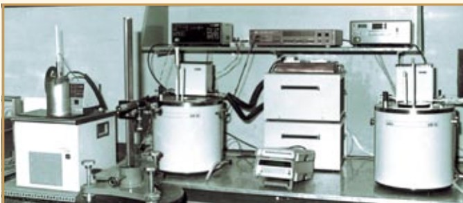
Experimental set-up for calibration of liquid-in-glass thermometers against standard platinum resistance thermometer (SPRT) using high stability temperature liquid baths in the range -90\text{ }^{\circ}\text{C} to 300\text{ }^{\circ}\text{C}
