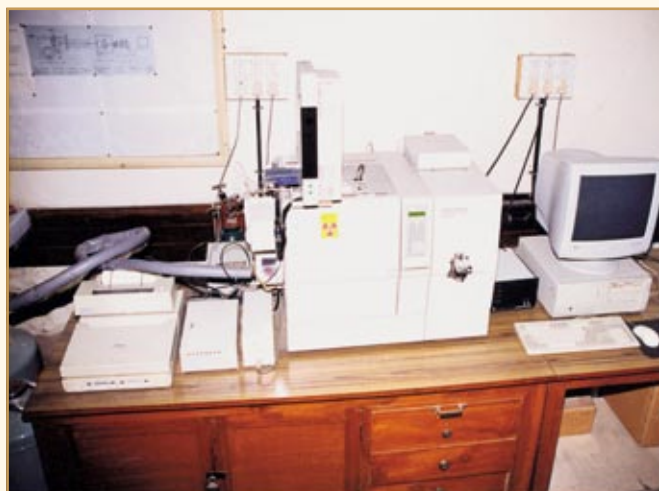
Gas Chromatography and Mass Spectrometer (GC-MS) facilities for trace inorganic and gas analysis
