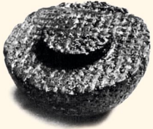
A view of the scaled down carbon-carbon composite nose tip developed at NPL
