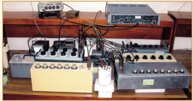
Kelvin double arm AC bridge established at NPL for build up scale of AC resistance standard from 1 \Omega to 1 M\Omega
