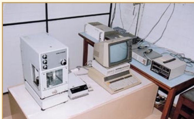
HK 1000 Mass Comparator is an automated computer controlled balance used to calibrate highest accuracy class 1 kg weights against the National Prototype Kilogram. Maintaining the traceability of the standard of mass at 1 kg level and its downward dissemination up to 1 mg is the main task of NPL
