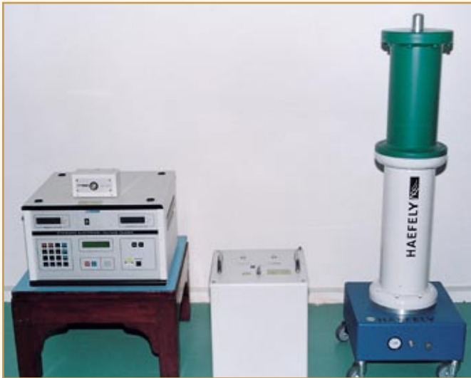
System for the calibration of Potential Transformers (PTs) of any voltage ratio from 110 V/110 V - 100 kV/100 V at 50 Hz
