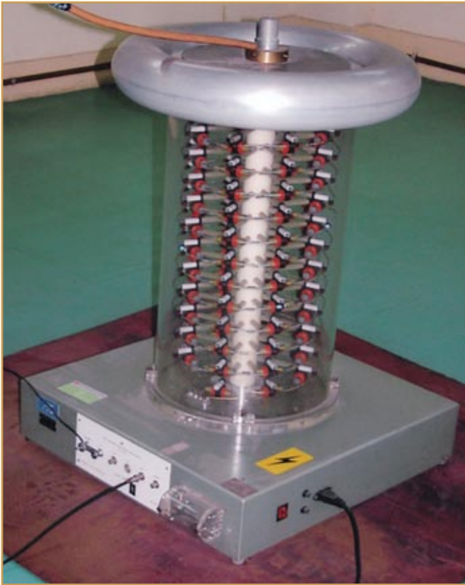
Resistive voltage divider, the primary standard of DC high voltage up to 100 kV, established in the year 2000
