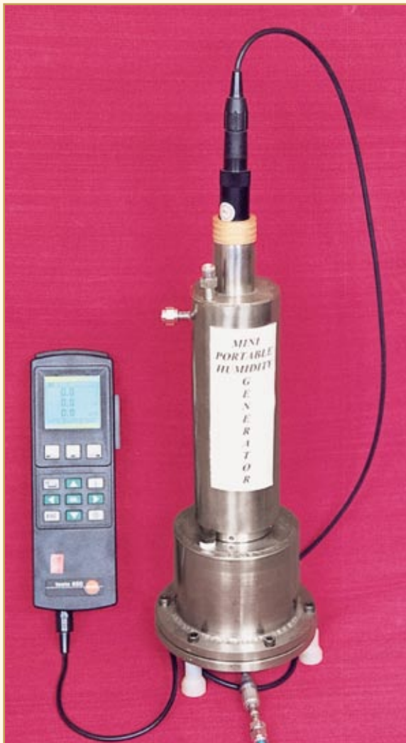
The first indigenous portable humidity generator based on two-pressure technique capable of generating Relative Humidity of 15% to 95%
