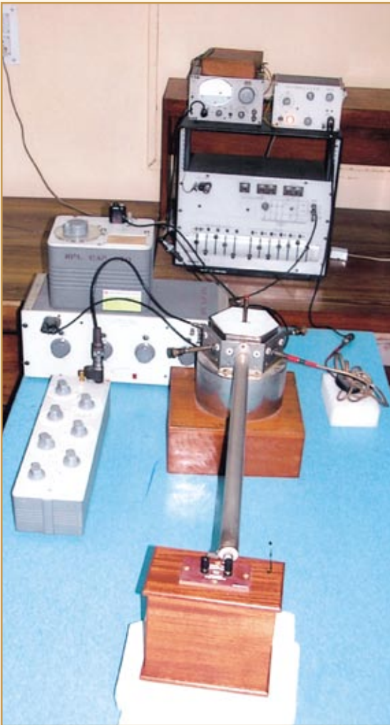
Maxwell - Wien Bridge, designed and fabricated at NPL for the realisation of inductance standard from capacitance and AC resistance
