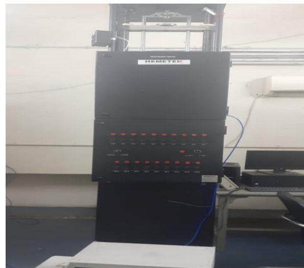
5 kN fully automatic dead weight force machine established at Force Metrology
