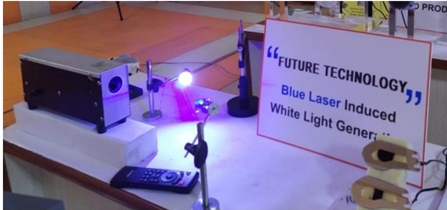
Demonstration of a blue laser induced phosphor coated white light prototype device developed at CSIR-NPL
