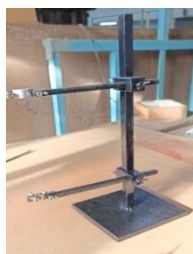
Fabrication of Stand for Holding Samples
