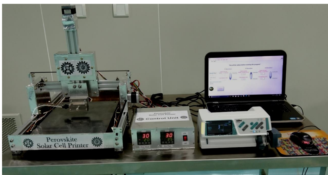
Photograph of the perovskite solar cell printer, which can print different layers of perovskite solar cells in 30 x 30 cm 2 area. The program, which controls the operation of the printer, is also shown in the laptop.
