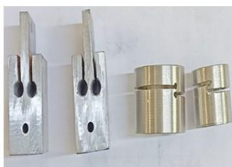
Fabrication of Hole Plates (Mild Steel)
