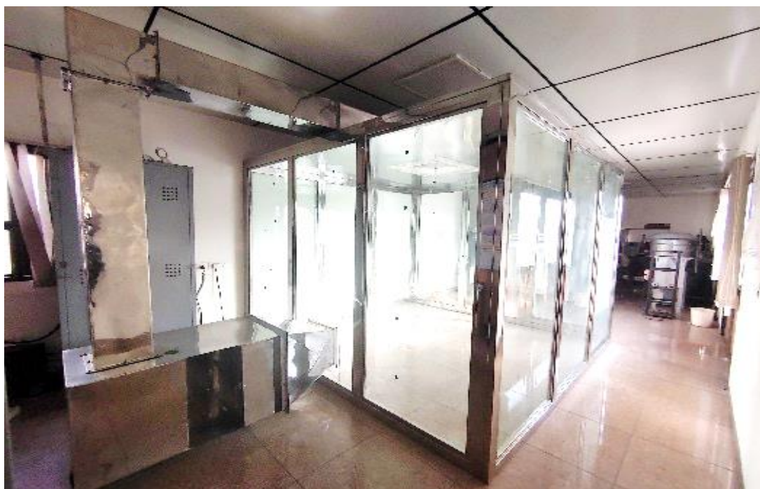
CADR test facility at CSIR-NPL
