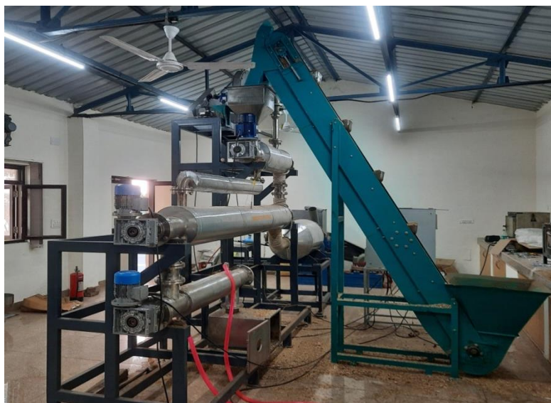
Indigenous torrefaction pilot for conversion of waste biomass in to biocoal
