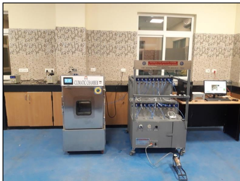
Final assembled system during testing as per OIML R-16
